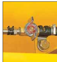
Fuel drain valve
