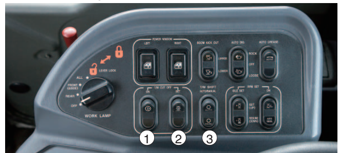
1:Transmission cut-off ON/OFF switch 3:Transmission shifting switch 2:Transmission cut-off set switch
