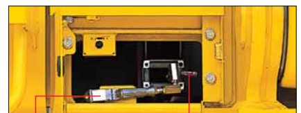
Grease gun The grease gun can be reached from ground level. Indicator
