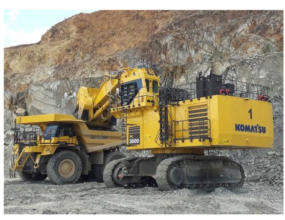
Even in confined work sites, you can maintain high production. The PC3000 is a powerful, versatile machine with advanced technology and a 16m<sup>3</sup> shovel and 16m<sup>3</sup> backhoe capacity, and the reach to fill 85-165 st trucks.
