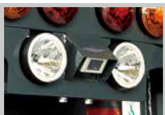
Stop, tail and turn signal lamps (LED)
