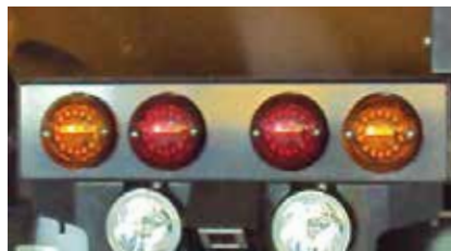
Stop, tail and turn signal lamps (LED)
